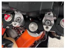
3. Install the bar risers to the triple clamp, using the two bolts you removed from the bar holders (note, as recommended in KTM repair manuals, use Loctite 243 or equivalent). You will see that one section of the bar risers is machined to allow the bolt head to sit flush with the top surface, this is where the existing shorter bolt goes. You can decide whether you want the bars to be offset forwards or backwards by the position of the shorter bolt in the triple clamps. See below.
