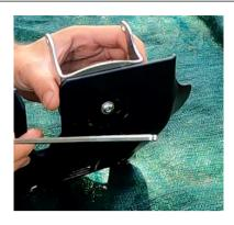
4. Now, mount the skid plate to the bike. Click the rear hook part of the skid plate over the frame, and lift the front up until the mount bracket holes line up with the holes in the frame (you may need to adjust the angle of the moutning bracket to get the alignment correct).
