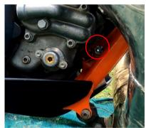
6. Tighten the bolt at the front which mounts the skid plate to the mounting bracket.
