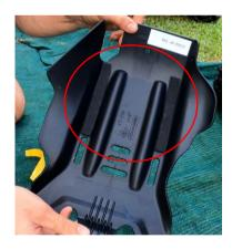
2. For skid plates that coming with a mounting bracket, install the nut clip so that the threaded portion point towards the folded tabs on the mounting bracket (the thread will face towards the gearbox).
