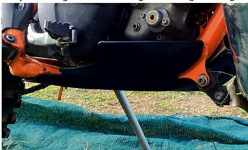
5. Using the bolts and nuts provided, fasten the mounting bracket to the bike frame (torque guide approx 10-12 N.m)
