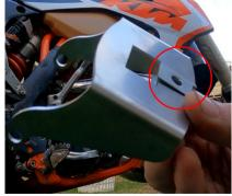
3. Using the bolt provided, install the skid plate mounting bracket to skid plate. Do not tighten the bolt, just leave it loose for now.
